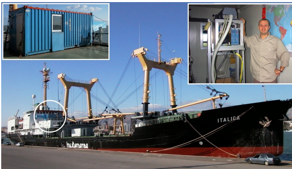
Figure 1: Main picture: RV Italica ; ELF and the ancillary instruments are housed in a container (inside the circle). Left insert: external view of the container; note on the right of the container the box accommodating the mirror for water surface observation. Right insert: internal view of the container; ELF is visible on the left of the operator.
